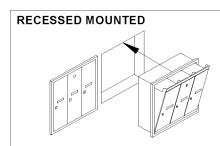
Units fit into a rough opening and are secured with mounting hardware through the back or side panels of the unit. Recessed units include a flanged collar which fits over the rough opening. (Hardware not included.)
