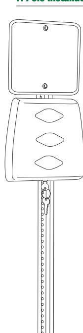
Using a post hole driver (not included), drive the sign post (C) approximately 15-18" into the ground. Make sure that the "hollow" or "recessed" side of the post is facing where you want the front of the unit to face. Use a level (not included) to ensure the pole is standing upright and will properly support the unit. Adjust if necessary.
